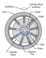
Radial-piston motors have a cylinder barrel attached to a driven shaft .The barrel contains a number of pistons that reciprocate in radial bores. The outer piston ends bear against a thrust ring. Pressure fluid flows through a pintle in the center of the cylinder barrel to drive the pistons outward. The pistons push against the thrust ring and the reaction forces rotate the barrel.
