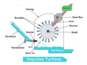
The pelton wheel or pelton turbine is tangential flow impulse turbine . The water strikes the bucket along the tangent of the runner. The Energy available at the inlet of the turbine is only Kinetic energy. The pressure at the inlet and outlet of the turbine is atmospheric. The turbine is used against high head.
