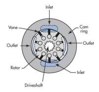
Vane motors have a slotted rotor mounted on a drive shaft that is driven by the rotor Vanes, closely fitted into the rotor slots, move radially to seal against the cam ring .The ring has two major and two minor radial sections joined by transitional sections or ramps. These contours and the pressures introduced to them are balanced diametrically.
