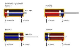
Double-acting cylinders are typically used in all applications where the thrusts and stroke lengths required are in excess of those available from single-acting cylinders. Small double-acting cylinders are also used for applications where positive end-of-stroke positions are required for both strokes.
