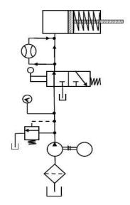
Above Figure shows that the control of a single-acting, spring return cylinder using a three-way two-position manually actuated , spring of f set direction-control valve(DCV). In the spring off set mode , full pump flow goes to the tank through the pressure-relief valve (PRV). The spring in the rod end of the cylinder retracts the piston as the oil from the blank end drains back into the tank . When the valve is manually actuated into its next position, pump flow extends the cylinder.
