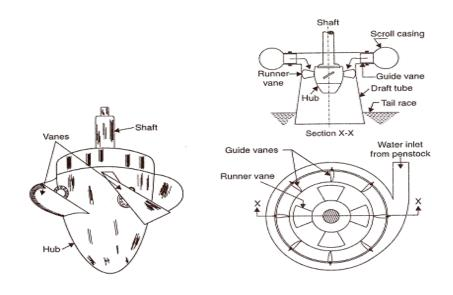
The Kaplan turbine is an inward flow reaction turbine, which means that the working fluid changes pressure as it moves through the turbine and gives up its energy. The desi combines radial and axial features.
