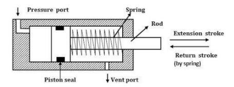
This cylinder only has a head end port & is operated hydraulically in one direction when oil is pumped into a part .It pushes on a plunger thus extend in git .To return or retract a cylinder. Oil must be released to reservoir. A plunger return either because of the of the weight of a load on from some mechanical force such as a spring.
