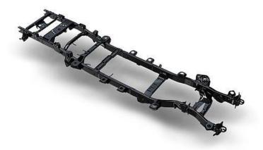
Heavy commercial vehicles such as trucks and buses mainly use the ladder frame structure. Some light commercial vehicles like pickup trucks also use the ladder frame. Tubular Frame:Some racing vehicles and All-Terrain vehicles use tubular frame design.
