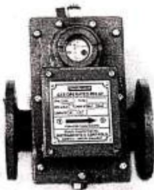
Buchholz relays are critical components of oil-immersed transformers rated above 500kVA. Usually what happens, transformer oil short circuits produce enough heat to cause the oil to break down into gases like methane, carbon monoxide, and hydrogen.
