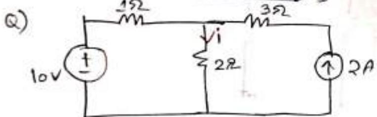
Find current in  $2\Omega$  resistor by using Thevenin & Norton's theorem.
