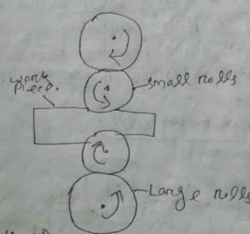
1 this consists of two small rolls for throwney reduction and two large backing rules to subport
