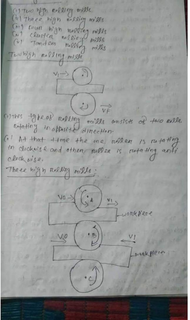
(1) Inthis case there are three walk one above the other at a times for single Pass two reals will be used. The rull direction will not be changed in this case. Cat The top two rulls will be used Bon Plast reduction and the sheet is shifted to the bottom two rules and Bunther neductionis done
