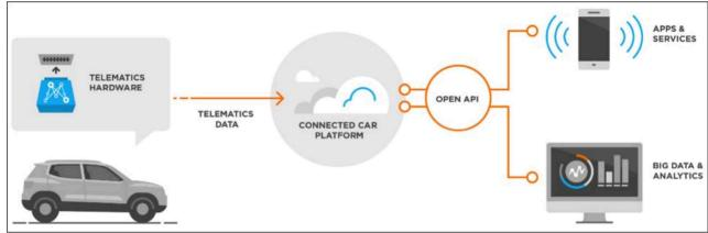
**Behavioral Data** — Mojio's telematics device gathers information about speed, steering, and braking inputs to determine driver's fatigue level and issue alerts. Long-term driving behavior data can also be used to help the user adopt a more fuel efficient driving style and calculate risk by insurance companies.
