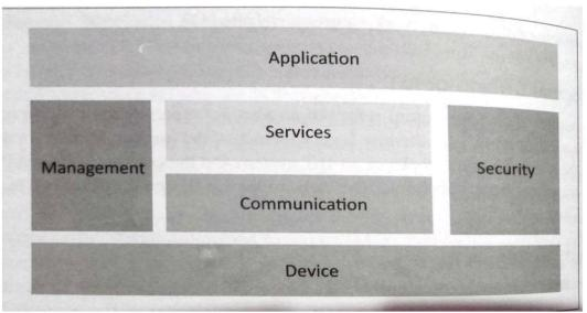
**Device:** An IoT system comprises of devices that provide sensing, actuation, monitoring and control functions.
