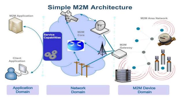
**Machine to machine (M2M)** is direct communication between devices using any communications channel, including wired and wireless.
